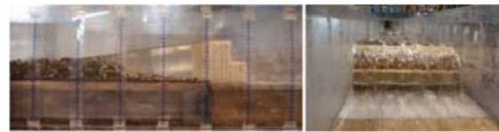
Figure 5. Closed check dam in the flume (view from the right-hand and downstream side).
